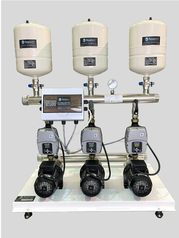
The Flowboost BASE Range is a Variable Speed Booster Set manufactured with Regulation 4/WRAS Approved horizontal multi-stage pumps and water cooled discharge mounted variable speed inverter drives with a vast array of features from the digital display, and available in single, twin and three pump configuration.
