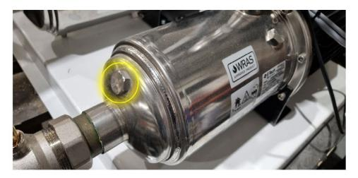
This operation should be repeated after around 10 minutes of operation as air can be brought through from the suction pipework or trapped between the pump impellors. Failure to do this may cause damage to the pump's mechanical seals and bearings. This in turn may cause noisy operation and leaks from the unit.
