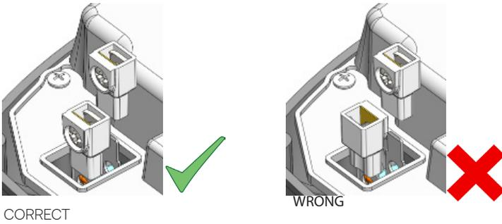
**CAUTION:** Insert the terminals, positioning them so that the cable tightening screws are not adjacent!
