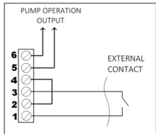
**Parameter "Aux. Con." = 4 – Combination with S inverter device.**
