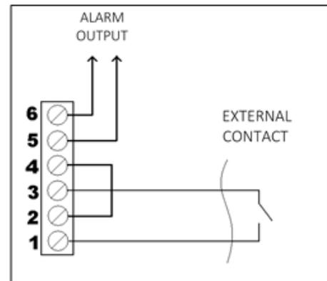
**Parameter "Aux. Con." = 3 – External enable and pump operation signal.**
