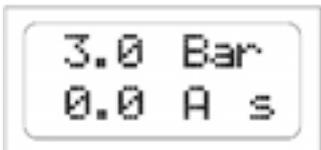
When the device is configured to operate as part of an alternating twin pumping unit, the bottom line shows the "master" or "slave" status by means of the letter "m" or "s".
