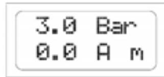
Main screen: during normal operation of the inverter, the display shows the device status. The top line displays the pressure measured in the system, while the bottom line shows the motor current absorption. In this screen, press and hold the key "+" to override pump operation also when there is no water, temporarily disabling the dry-running protection to enable the pump to be filled.
