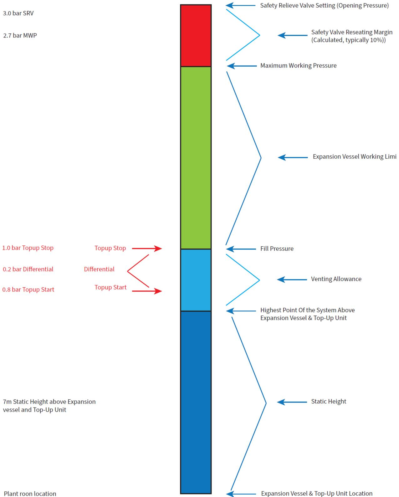
A typical venting allowance is 0.3 bar, added to the static height to give the cold fill pressure. The Differential setting represents the allowable pressure loss before the pump activates and restores the cold fill pressure. The Differential setting must not be greater than the system venting allowance.
