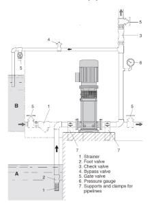
Secure all pipes to their rests close to the pump and connect them so that they are not subjected to stress and do not transmit vibration or flexion strain to the pump (see fig.3).
