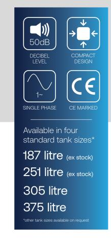
Introducing the **flowpac** Compact 1F.DT CAT5 Packaged Booster Set range, available as a single pump only with 4 standard tank sizes. All tanks have a footprint of 670mm x 650mm making the units ideal for small plant rooms. Suitable for single or multiple outlets.
