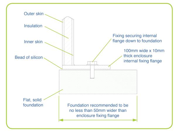
For the successful installation of Flowstore GRP Housing Enclosures, please ensure the following requirements are met:
