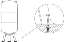
Fig. 4 Example of floor installation
