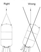
Fig. 3 Lifting the tank
