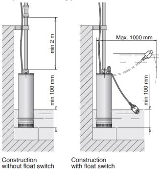
The pump can be rested on the flat bottom surface of a tank. When sand or slime deposits are expected to form, mount the pump on a surface raised from the bottom level so that abrasive matter is not lifted.
