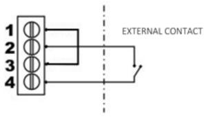
according to the Pmax pressure value, while when the external contact is closed the device shall adjust the pump speed according to the Pmax2 value.
