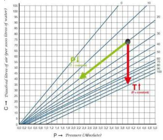
The Flowmat (PHP) system with its pressure drop design allows dissolved air to be released from the system water. This is enhanced by a cartridge of patented PALL rings in the inlet stream to the vessel. The released air is allowed to vent out of the vessel via and automatic air vent on the top. The air vent is also fitted with a non return valve to prevent air being drawn back into the system.
