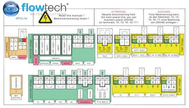
SPC Wiring - 230v - Single Phase - 50 Hz (SPCx-lw)
