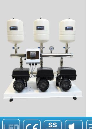
The Flowboost PRIME Range is a Variable Speed Booster Set manufactured with Regulation 4/WRAS Approved horizontal multi-stage pumps and pump mounted variable speed inverter drives with a vast array of features from the digital display, and available in single, twin and three and four pump configuration.
