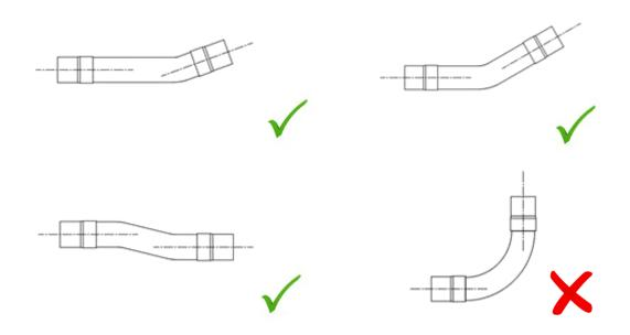
We supply various size flexible connections from 1 ¼" to 4" to suit our manifold sizes. The smaller sizes are more pliable but still should not be used as elbows. The bigger sizes are very rigid and may not bend very easily. As with any flexible connector, if they are overly bent through awkward angles they will kink and become unusable, as the bore will be reduced and may not allow the required amount of flow through the pumps or to the system.
