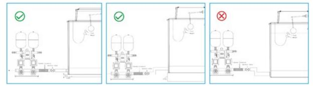
The purpose of a tank plinth or base is to support the tank but also to provide an elevated starting point where water can reach the booster equipment under gravity. Most tank bases will be around 150mm in height or higher if required for access to bolts underneath the tank.
